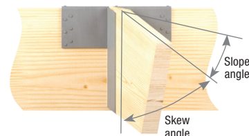
Typical HLBH hanger sloped down, skewed right, center flush shown
